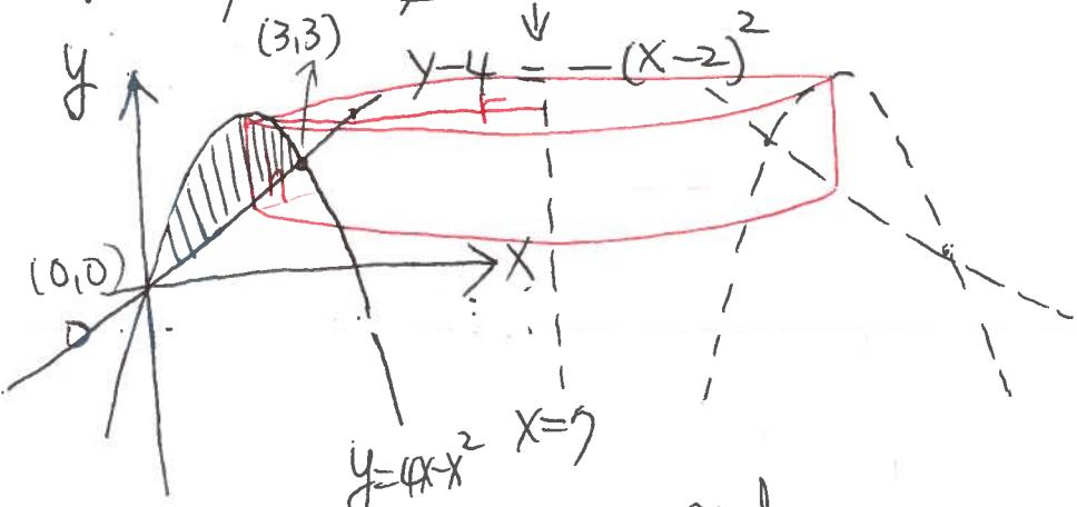
$$\begin{aligned} r &= 7-x \\ h &= 4x-x^2-x = 3x-x^2 \\ x &\in (0, 3) \end{aligned}$$
